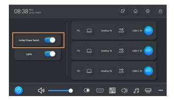
The "Unified Power Switch" is a power switch controlled by the NDP100. It enables one-touch activation or deactivation of devices connected to the Digital Podium such as Built-in PC, Gooseneck microphone, Tabletop power outlets, etc.
