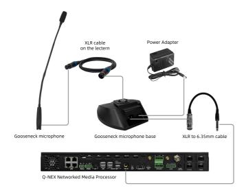
The NDP100 is equipped with a gooseneck microphone suite, powered by a Power Power connected to the base.
