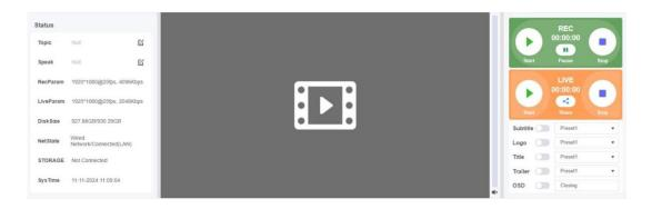
The largest screen on the home page is the movie screen, which is the composite screen for recording/live streaming. In manual mode, you can switch the movie screen by double-clicking or dragging the standby screens (video preview small windows) below.
