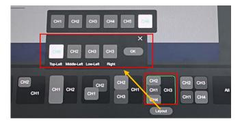
Select the four-screen display mode, click "Layout", and a pop-up window will appear with the video channel arrangement of the four screens. Click one of the video channels, and a pop-up window will appear with all six video channels (video sources). Select the video source required for the screen position, for example, "CH6". After all settings are completed, click "OK".
