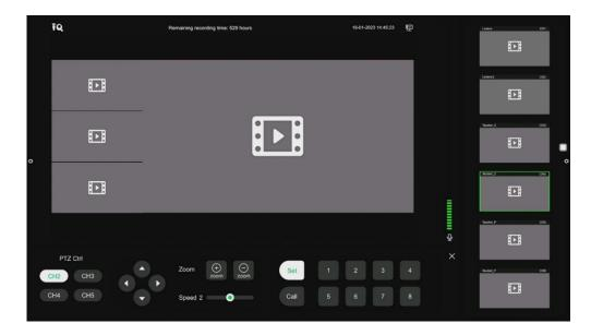
When the director mode is switched to "manual" mode, the director can set and activate preset positions for PTZ cameras of different channels through the PTZ Control area, as well as to perform operations such as zooming in and out.
