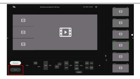
: Buttons for setting screen layout in manual mode; they represent single screen, dual screen PIP, dual screen dual split screen, triple screen, quad screen, and all screens.
