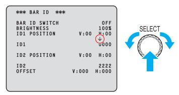
2. Turn the [SELECT] dial to move the cursor to position where a character is to be input, and then press the [SELECT] dial.
