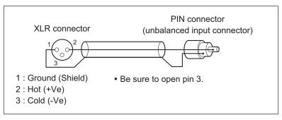
Some commercially available conversion connectors and conversion cables have pin 3 shorted to pin 1.
