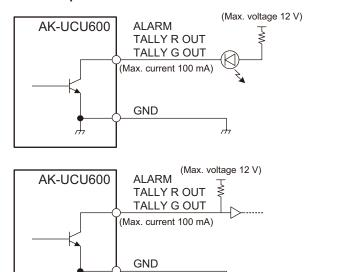
Withstand voltage: 12 V DC max. Power current: 100 mA max.
