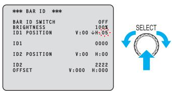
When the setting value is confirmed and the flashing stops, you can move the cursor.
